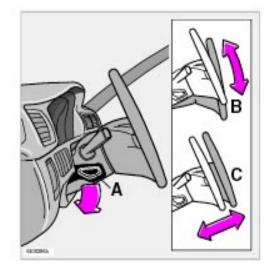
Pull down the lever (A) to adjust height (B), or reach (C)
